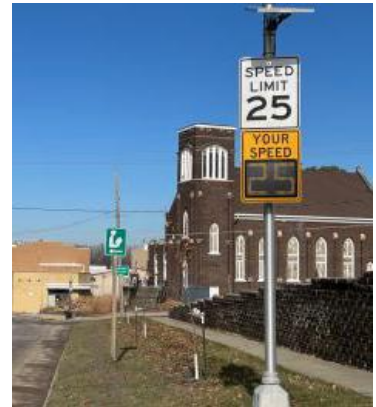
Figure 25 Speed feedback sign with posted speed limit and display of driver's speed. Source: IOWA DOT
