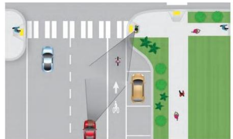
Figure 8 Example of a curb extension with restricted parking. Source: PEDSAFE
