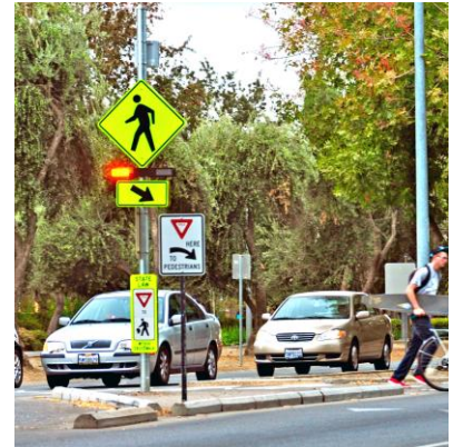
Figure 23 Rectangular Rapid Flashing Beacon in use at a crosswalk. Source: www.pedbikeimages.org / Lara Justine
