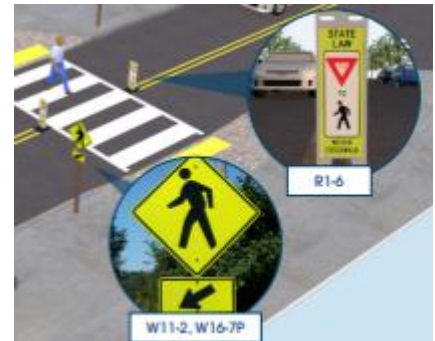
Figure 5 Example of crosswalk visibility enhancements. Source: FHWA
