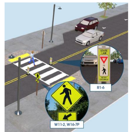
Figure 6 Example of high visibility crosswalk. Source: FHWA
