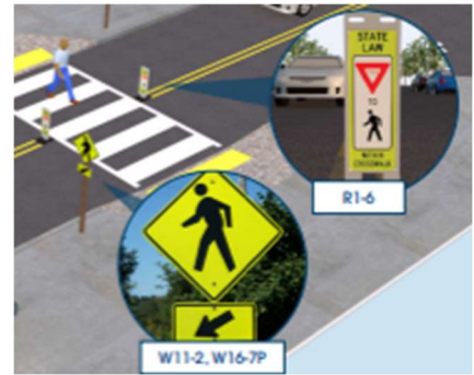
Figure 5 Example of crosswalk visibility enhancements. Source: FHWA
