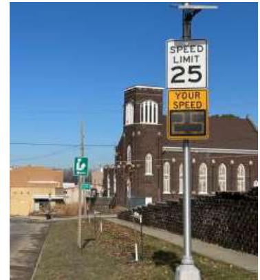
Figure 25 Speed feedback sign with posted speed limit and display of driver's speed. Source: IOWA DOT
